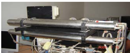
Fig. 8. Photo of the reverse osmosis desalination system
