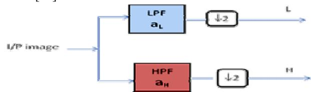
Fig. 2. Two-channel Filter Bank
