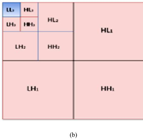
Fig.3.(a)2D Discrete Wavelet Transform (DWT) (b) Pyramidal Structure of Wavelet Transform
