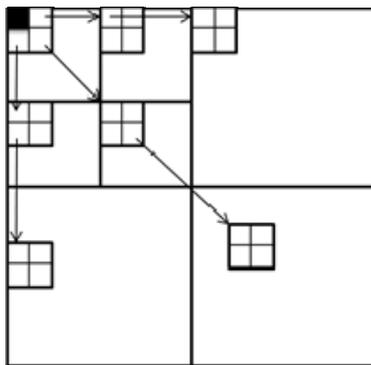
Fig. 7: Parent- offspring in 2D SPIHT.
