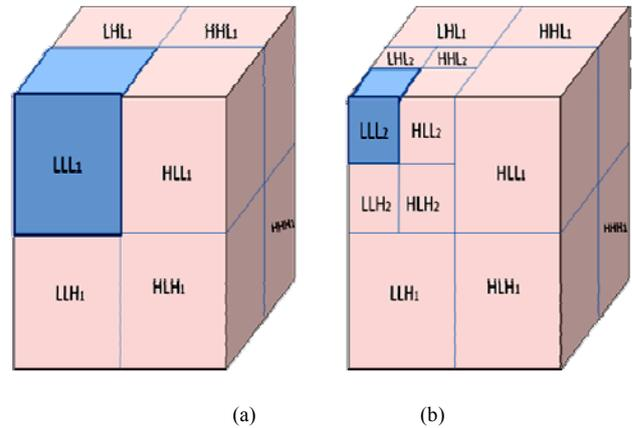
Figure 4 (a) 3D, 1 level wavelet decomposition, (b) Second level decomposition.
