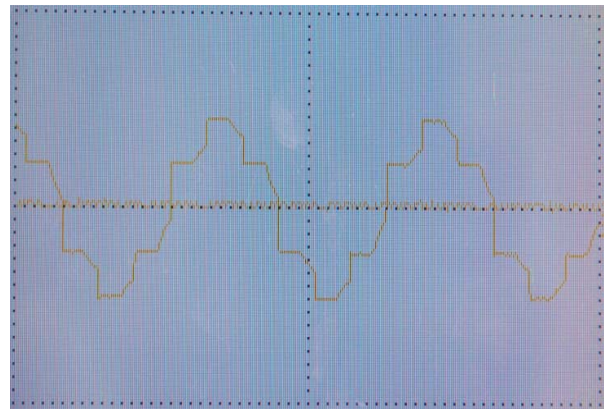
Fig.22. Output line voltage waveform for phase B
