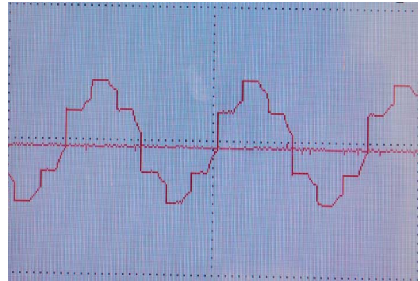
Fig.20.Output line voltage waveform for phase R
