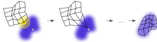
Figure 2: An illustration of the training of a SOM. The blue blob is the distribution of the training data, and the small white disc is the current training sample drawn from that distribution. At first (left) the SOM nodes are arbitrarily positioned in the data space. The node nearest to the training node (highlighted in yellow) is selected, and is moved towards the training datum, as (to a lesser extent) are its neighbours on the grid. After several iterations the grid tends to approximate the data distribution (right).
