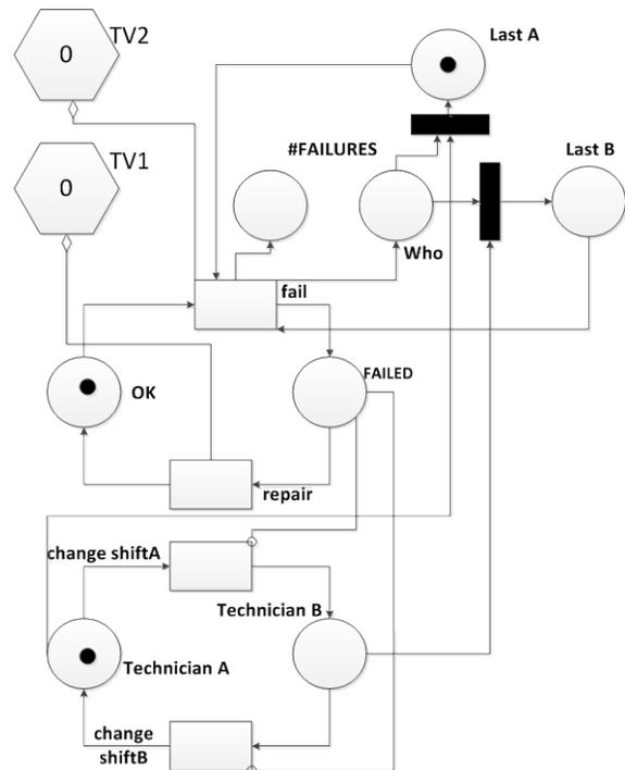
Fig. 6. Basic Petri net + factor (a) model of the example
