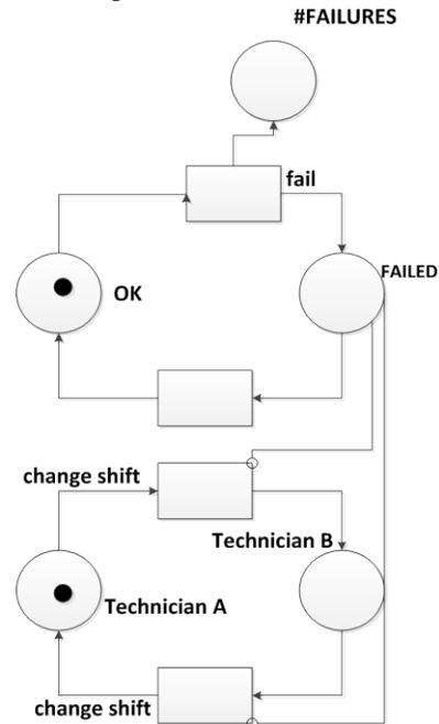
Fig. 4. Basic Petri net + factor (a) model of the example
