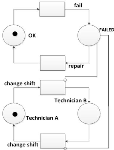
Fig. 2. Basic Petri net model of the example
