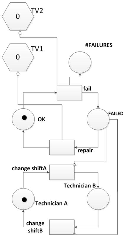
Fig. 5. Basic Petri net + factors (c,d) model of the example
