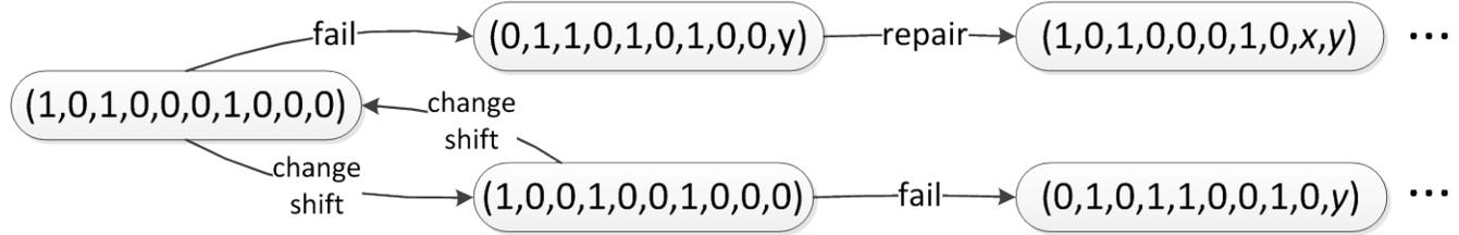
Fig. 7. State-transition diagram of the unbounded Petri net model from Figure 3
