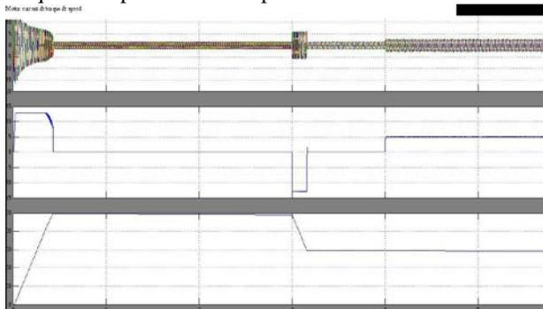
Figure9.Input current, Generated Torque and Rotor Speed waveforms of VCIM with PWM Rectifier
