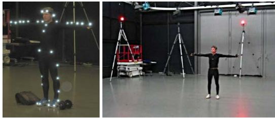
Fig.2. Optical motion capture system based on retro-reflective markers attached to the actor's body.
