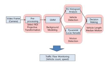
Fig. 2 Automatic vehicle detection and counting algorithm.
