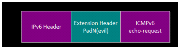
Figure 1.3.: Covert Channel inside the Padding of an Extension Header.
