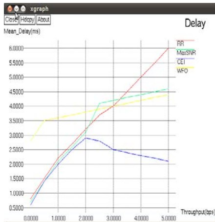
Fig 4.2 The delay is shown in this graph. In the X-axis Throughput is taken. Y-axis Mean delay is taken. This graph clearly shows the mean delay is decreases in CEI (coverage extension based on incentive scheduling) compared to the existing algorithms.
