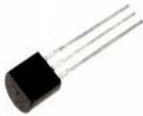
Fig 4.1: LM 35 Temperature sensor.
