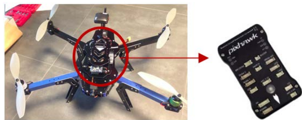
Fig. 3 3D Robotics quadcopter and its Pixhawk
