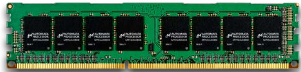
Fig. 8 Eight Micron AP chips forming one rank.
