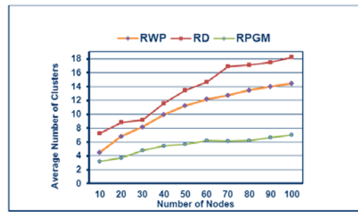
Fig. 5 Average number of clusters vs. number of nodes for speed 30 m/s (scenario 1).
