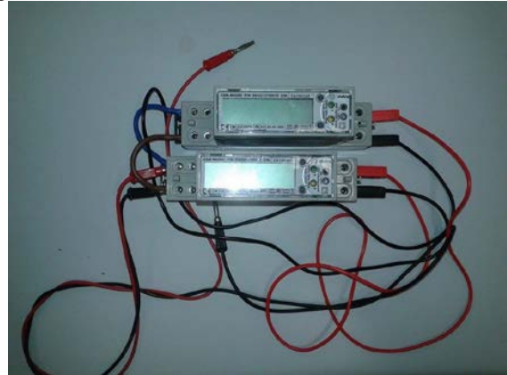
Fig. 2. Power network analyzer used in the experiments
