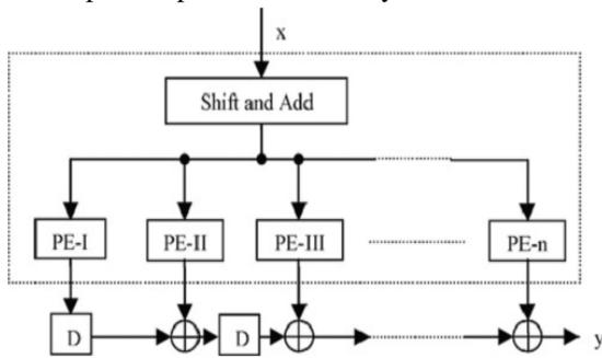
Figure-2: Transposed direct form of an FIR filter
