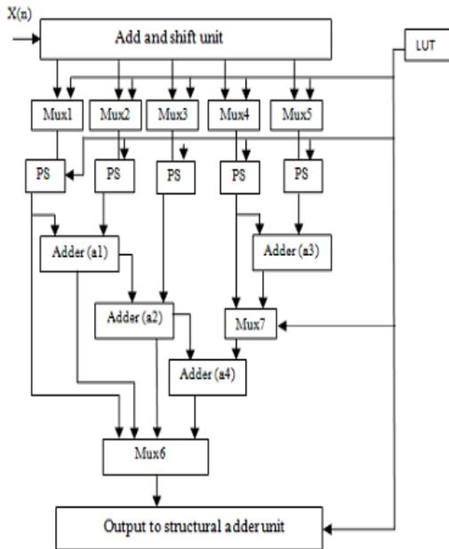
Figure-4: Architecture of PE for PSM
