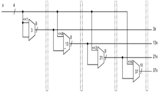
Figure-1: Block Diagram of Minimized Adder Graph
