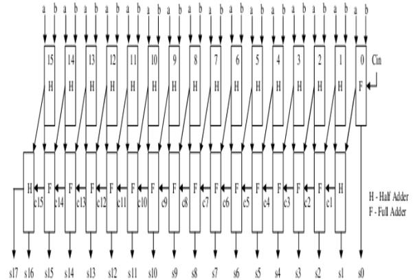
Figure-5: Block Diagram of 16-bit Carry Save Adder
