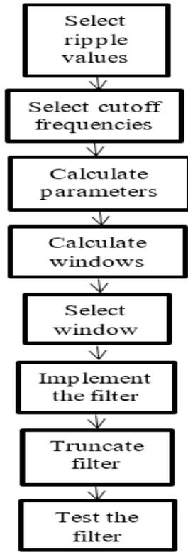
Fig. 2 The proposed FIR filter approach.
