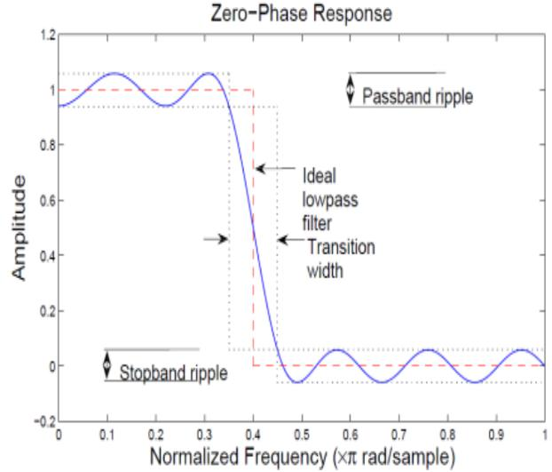
Fig. 1 Typical normalized low pass filter.
