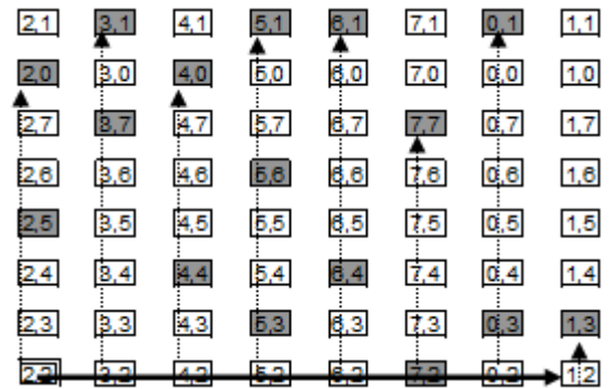
Fig. 2 Message multicast routing by using T2W algorithm
