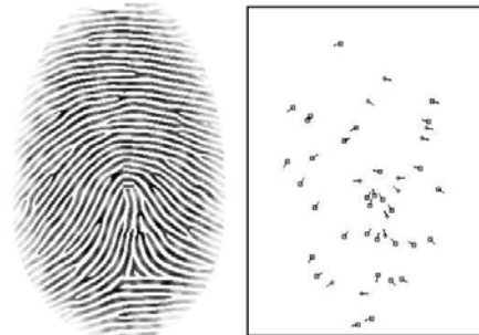
Figure 5: Grey scale fingerprint and extracted minutiae points
