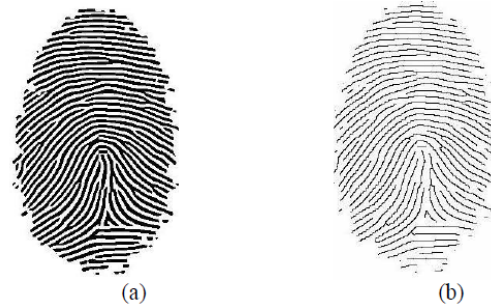
Figure 4: Binarized image and thinning image
