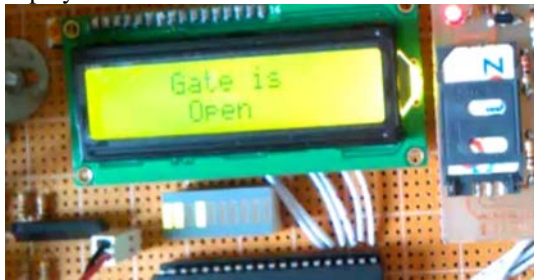
Fig. 6.Gate is opened for authorized visitor
