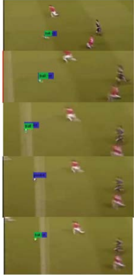
Figure 7. Estimating ball movement direction in seven consecutive frames by using Lucas Kanade and crossing overlap with the ground line.
