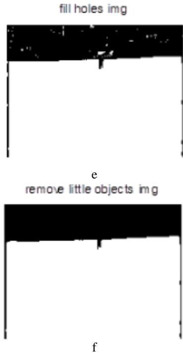
Figure 1. How to estimate grass border, a: input image, b: hue transform, c: hue histogram and the amount of grass hue, d: thresholding on hue page, e: filling the bubbles in the grass, f: selecting the largest area and removing unwanted margins.
