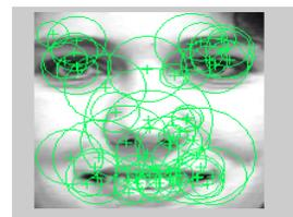
Figure 4. Features extracted from test image shown in green color
