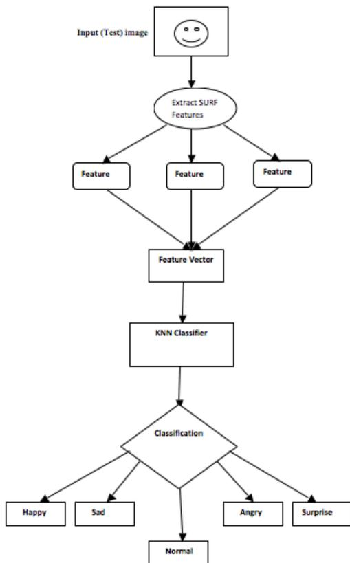
Figure 7. Complete flow of algorithm
