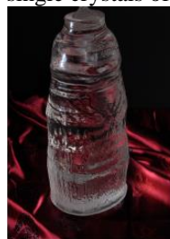
Sapphire Crystal grown in a Boule
