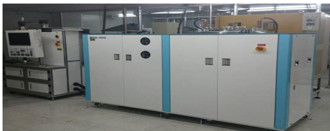
SUNPHIRE's 100 KG KY SAPPHERE GROWER / FURNANCE
