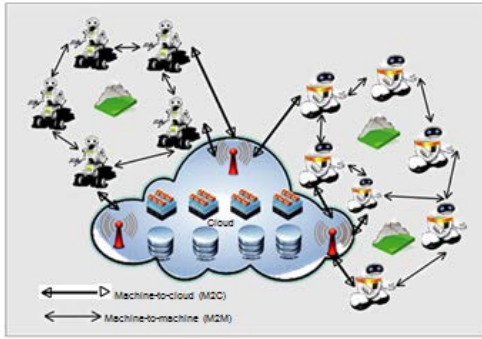
Figure 2. Cloud Robotics: robots are interconnected via M2M/M2C communications, sharing their resources and accessing to remote cloud resources.
