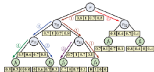
Fig. 3. An example of the tree-based index with the document collection F = \{f_i | i = 1, \dots, 6\} and cardinality of the dictionary m = 4 . In the construction process of the tree index, we first generate leaf nodes from the documents. Then, the internal tree nodes are generated based on the leaf nodes. This figure also shows an example of search process, in which the query vector Q is equal to (0, 0.92, 0, 0.38) . In this example, we set the parameter k = 3 with the meaning that three documents will be returned to the user. According to the search algorithm, the search starts with the root node, and reaches the first leaf node f_4 through r_{11} and r_{12} . The relevance score of f_4 to the query is 0.92. After that, the leaf nodes f_3 and f_2 are successively reached with the relevance scores 0.038 and 0.67. Next, the leaf node f_1 is reached with score 0.58 and replace f_3 in RL_{list} . Finally, the algorithm will try to search subtree rooted by r_{12} , and find that there are no reasonable results in this subtree because the relevance score of r_{12} is 0.52, which is smaller than the smallest relevance score in RL_{list} .
