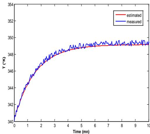
Fig. 8 Estimation of the temperature  $T$  in the presence of a measurement noise
