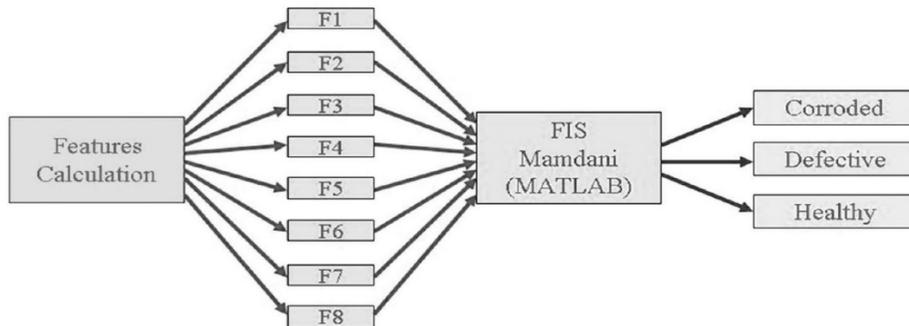
Figure 10: FIS structure related to the classifier of defects. FIS can be developed using MATLAB program
