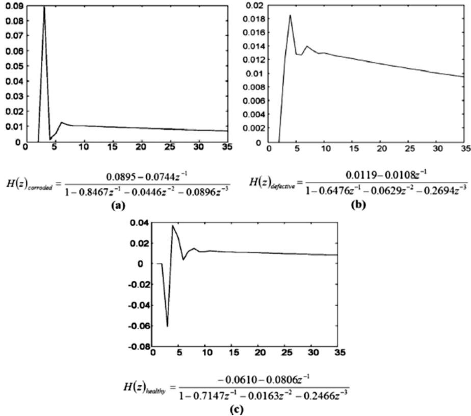
Figure 8: impulse response and the obtained transfer functions of a) corroded metal, b) defected metal and c) healthy metal.
