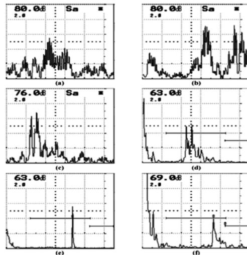
Figure 7: the different kinds of data related to the a) holes, b) light deterioration, c) gaps, d) joints, e) cracks, and f) resulted from partial melting
