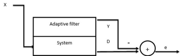
Figure 4: Diagram block of comparative filter
