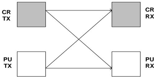
Fig. 1 Point-to-Point communication links in CRN
