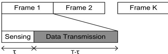
Fig. 2 Single-slot time division spectrum sensing framework.
