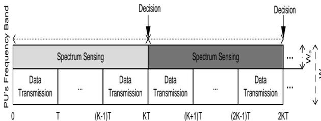
Fig. 5 Throughput oriented frequency division spectrum sensing framework
