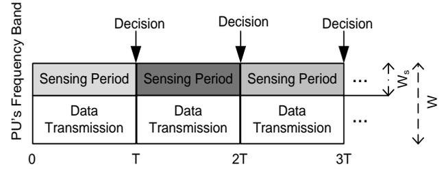
Fig. 4 Delay oriented frequency division spectrum sensing framework
