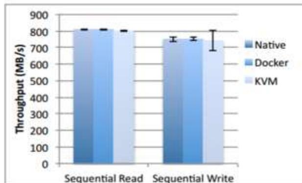
Fig. 8 Sequential I/O throughput (MB/sec) [3].
