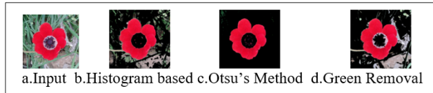
Figure 3: Threshold-Based Segmentation for Papaver Species
