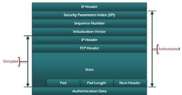
Fig. 6 ESP Header in Tunnel Mode
