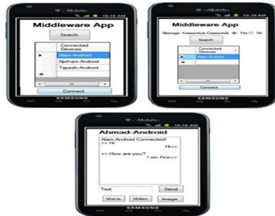
Fig. 7. Middleware implementation using android application
