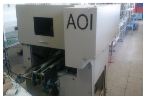
Figure (16). The built AOI machine
