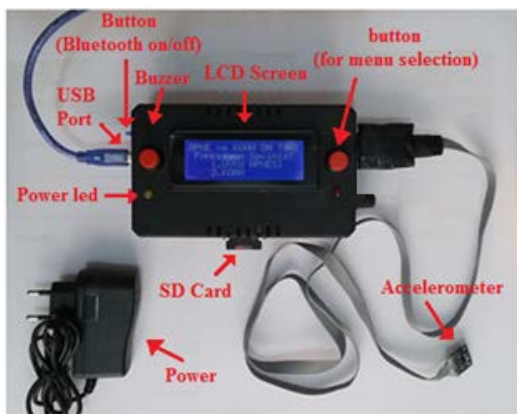
Fig. 6 Developed diagnostic device and equipments
