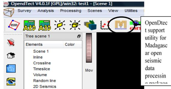
Fig. 9 The icon ‘M’ noted by the circle indicates the OpenDtect-Madagascar support utility located on the main page of OpenDtect software
