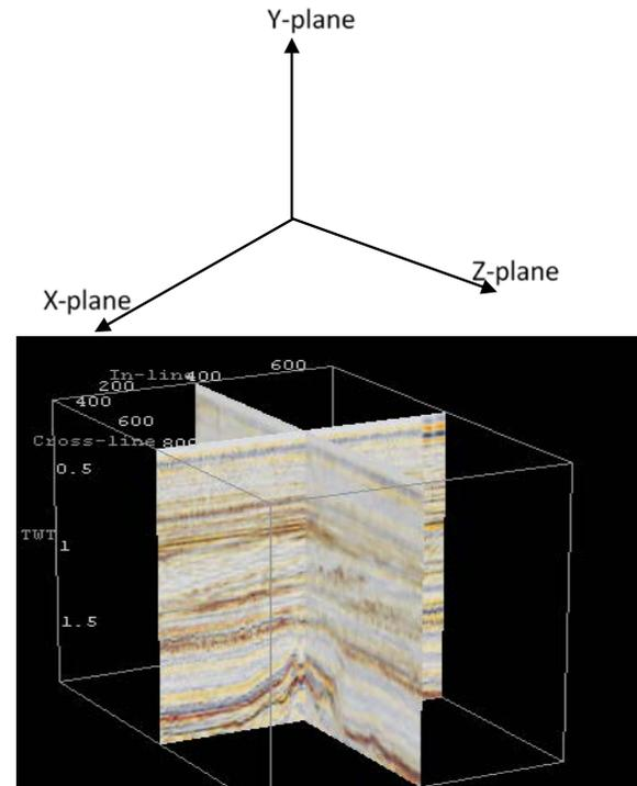
Fig. 1 The x, y and z plane which represents the horizontal, vertical and depth surface respectively
