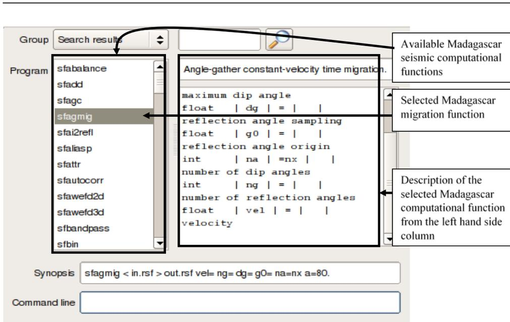
Fig. 10 The scroll down list of available Madagascar computational functions supported by OpenDtect is apparent on the left hand-side column
