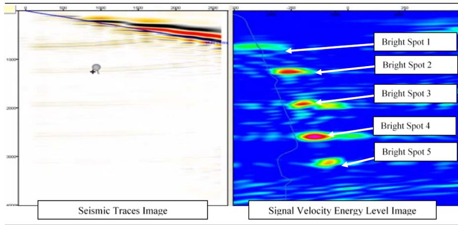
Fig. 5 Image on the left indicate the seismic traces where by image on the right is the signal energy level. Bright spot shows the high energy values [7].
