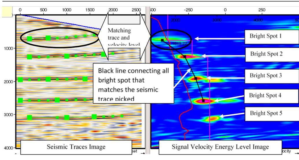
Fig. 6 Image on the left indicate the seismic traces where by image on the right is the signal energy level. Bright spot shows the high energy values [7].
