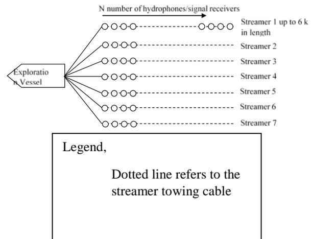
Fig. 2 Signal receiver deployment layout viewed from top during a marine geological mapping operation to acquire 3D seismic data
