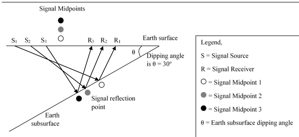
Fig 8 Figure shows an multiple signal reflection point a 30° Earth subsurface dipping angle
