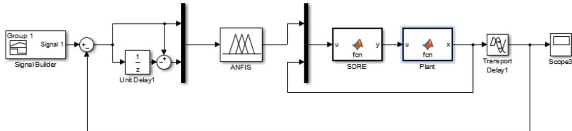
Fig. 4 The overall closed-loop structure of diabetes control in the presence of SDRE controller neuro-fuzzy network for adaptive weighting
