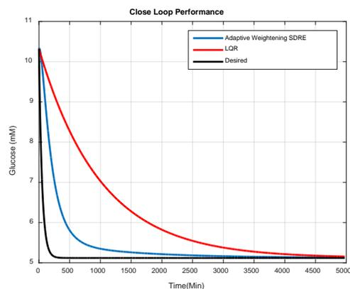
Fig. 5 Closed-loop response of controlled system (glucose variations), comparison of proposed method against LQR
