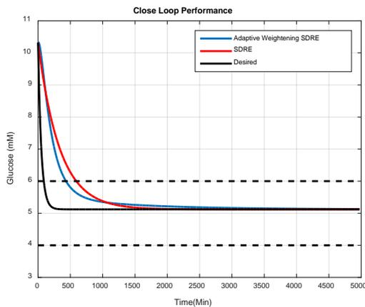
Fig. 7 Closed-loop response of controlled system (glucose variations), comparison of proposed method against SDRE
