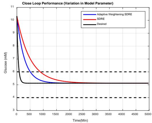
Fig. 8 Closed-loop response of controlled system (glucose variations in the patient), comparison of the proposed method against SDRE if there is 10% variation in  $\gamma$
