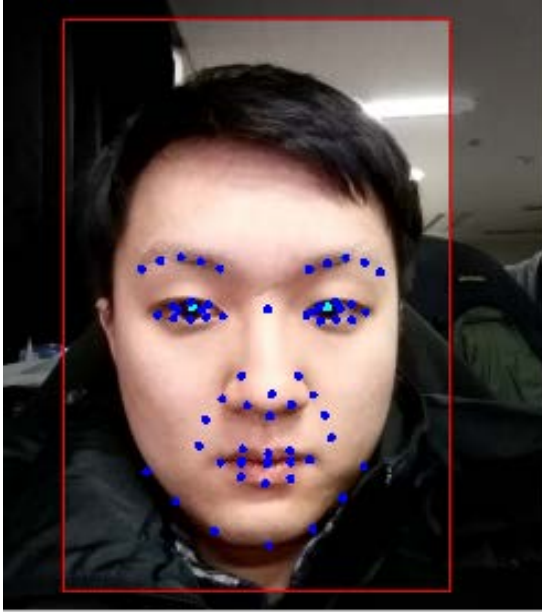
Fig. 2 Laxuad Face SDK with 66 facial feature points.
