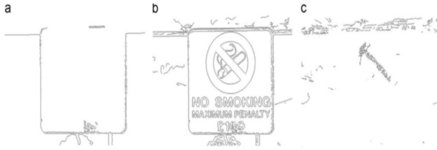
Fig. 10 An example of edges extracted from different channels: (a) Gray channel. (b) L channel. (c) Detail channel. [22]
