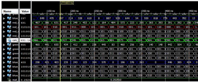
Fig. 6 Waveforms for RGB to YCbCr and YCbCr to RGB Conversion
