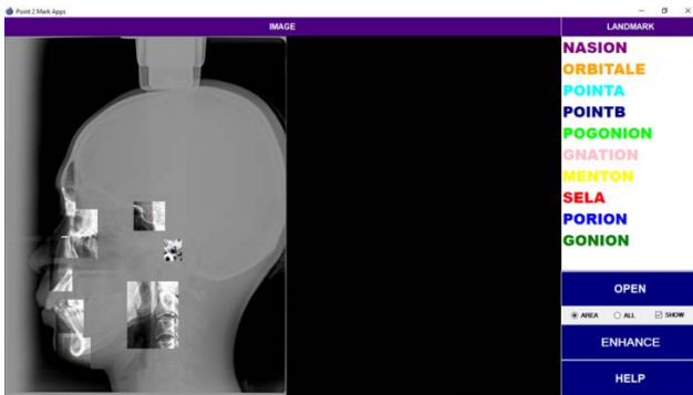
Fig. 3 The marked landmarks and ROI position
