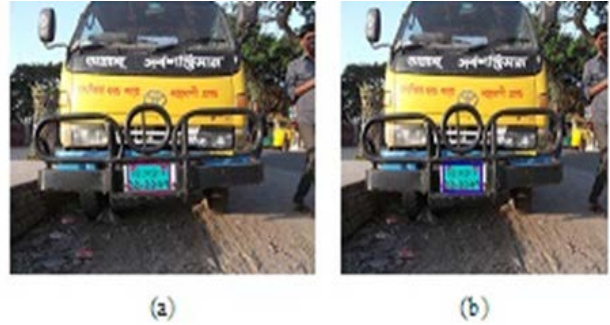
Fig. 4 (a) Selected contour (marked by pink color), (b) the rectangle over the contour (marked by blue color).
