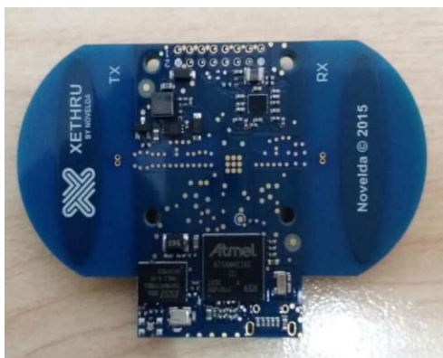
Fig. 3 Respiration Detection Hardware Module
