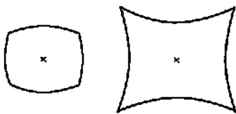
Fig. 3 Effect of radial distortion on image geometry
