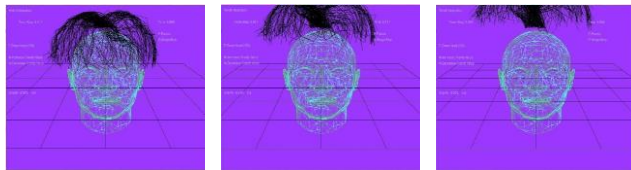
Fig. 11 Animation frames when upwards directed wind effect is applied onto hair model. a) Animation frame at 5.685 s. b) Animation frame at 6.417 s. c) Animation frame at 6.884 s.
