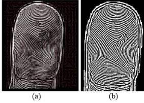
Fig. 4 Results after applying different steps on normalized image: (a) Ridge orientation, (b) Image binarization.
