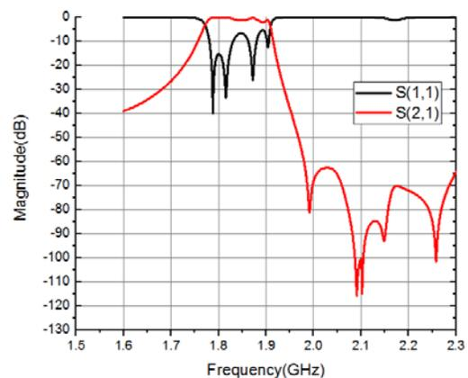
Fig. 7. Ceramic waveguide Filter-II (HFSS Simulation)
