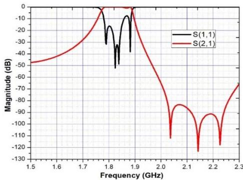
Fig. 5 EM simulated response of the Filter-I
