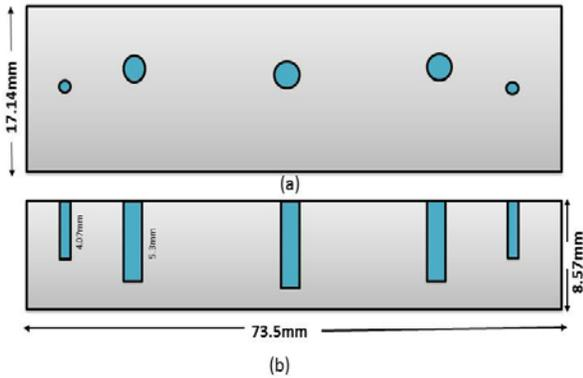
Fig. 4 Physical layout of the Filter-I (a) Top view (b) Side view
