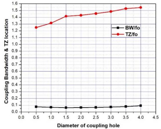
Fig. 3 Coupling bandwidth and Tz location variation with respect to hole diameter
