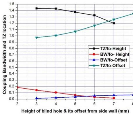
Fig. 2 Coupling bandwidth and Tz location variation with respect to hole height and its distance from side walls.
