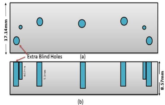
Fig. 6 Physical layout of the Filter-II (a) Top view (b) Side view
