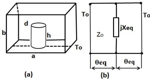
Fig. 1 resonating coupling hole (i) Physical layout (ii) equivalent circuit.
