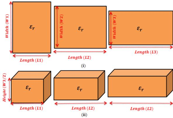
Fig. 1 Three different width resonators with same fundamental frequency
