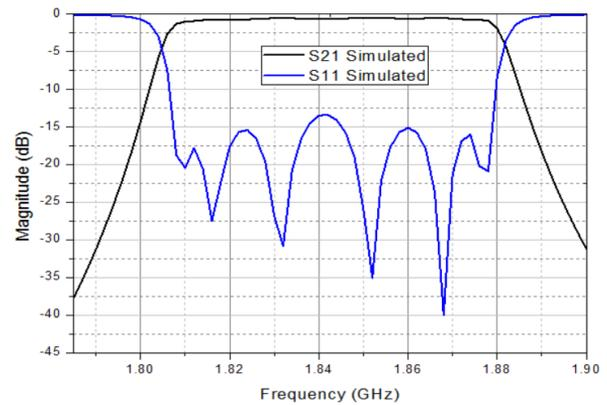
Fig. 3 simulated Passband response of a filter with first configuration.
