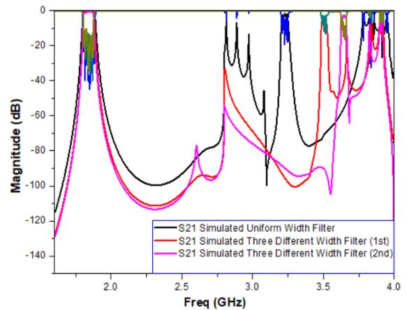
Fig. 8 Comparison of stop band performance of both three different width ceramic resonator filters with uniform width ceramic filter
