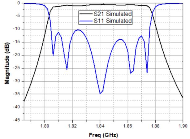
Fig. 6 Simulated Pass band response of three different width ceramic waveguide filter in second configuration
