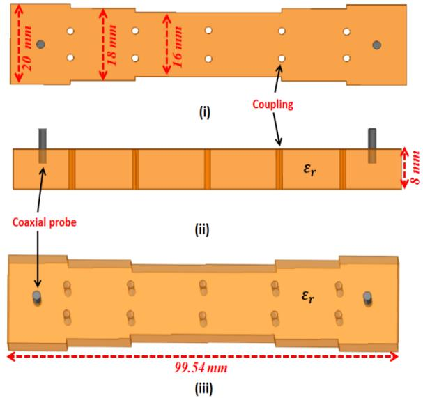
Fig. 2 physical layout of monolithic ceramic waveguide filters with three different width resonators in first configuration(i) Top view (ii) Side view (iii) 3D view
