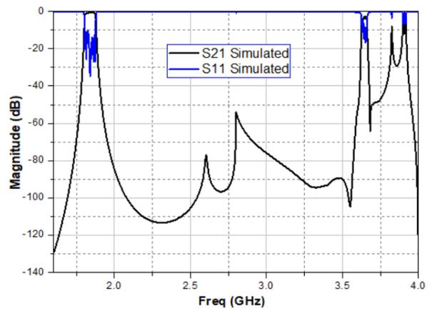
Fig. 7 Simulated broadband response of three different width ceramic waveguide filter in second configuration
