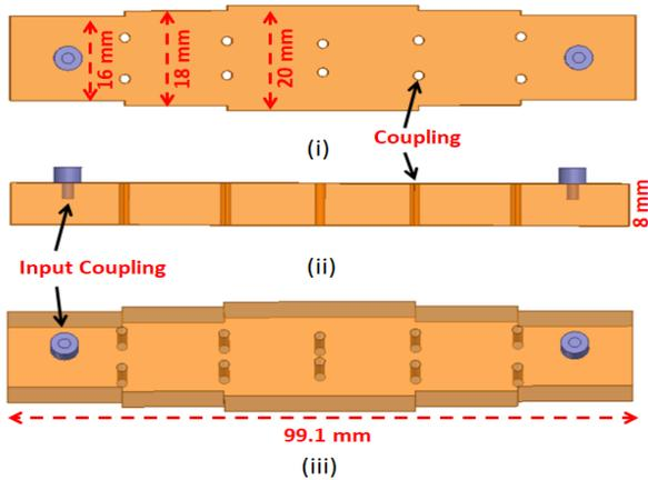
Fig. 5 physical layout of monolithic ceramic waveguide filters with three different width resonators in first configuration (i) Top view (ii) Side view (iii) 3D view
