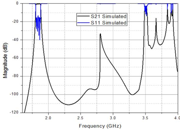
Fig. 4 Simulated broad band response of three different width ceramic waveguide filter in first configuration
