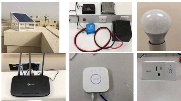
Fig. 3 Photograph of connected parts: solar panel, battery charger, light, Wi-Fi router, smart plug and switch.
