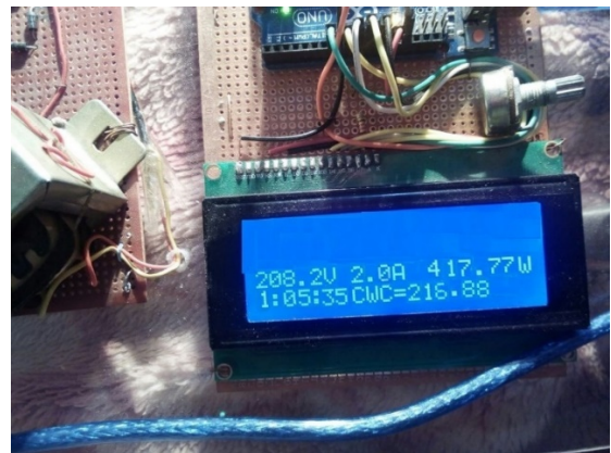
Fig. 11 Active Power Load of TV (Television) Smart Hardware Module
