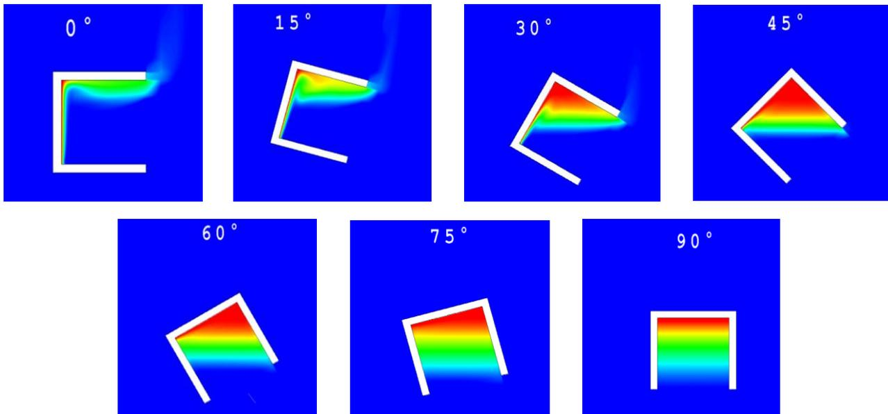
Fig. 3. Temperature contours of cavity at wall temperature  $T_w = 340^\circ K$  for various Degrees of Inclination.
