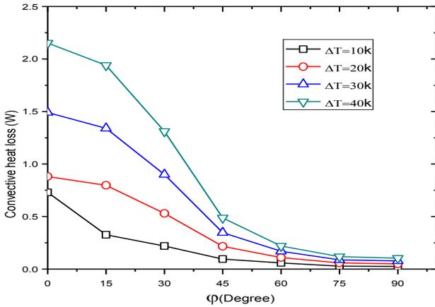
Fig. 4. Variation of the Convective heat loss  $Q_c$  with the cavity inclination angle  $\phi$
