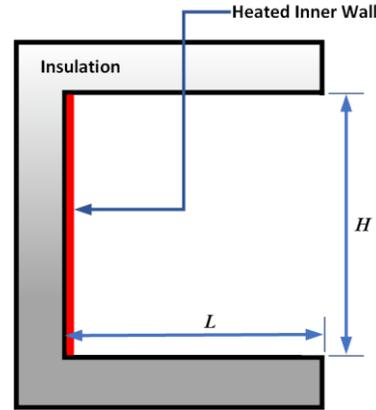
Fig.1. Open Cavity Structure.
