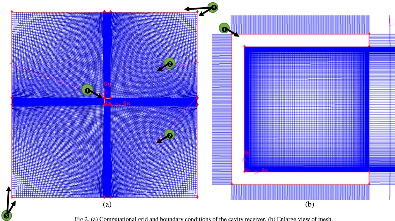
Fig.2. (a) Computational grid and boundary conditions of the cavity receiver. (b) Enlarge view of mesh. Labels: ❶ Cavity Receiver, ❷ Extended Domain, ❸ Pressure Inlet
