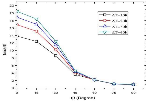
Fig. 5. Variation of the Average Convective Nusselt Number  $\overline{Nu}_c$  with the cavity inclination angle  $\phi$
